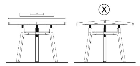
Make sure that the spindles are extended the to the same height
