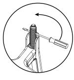
Turn the spindles untill the hole is approximately 1cm above the top of the leg
